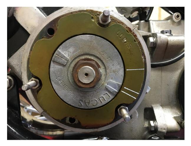
My bike is fitted with a 38MM carb (possible factory upgrade based on the bikes documentation). It is not known if the bike has Peter Green porting. The Lumenition ignition was strobed at an estimated 33Deg BTDC prior to dismantling based on these markings.
