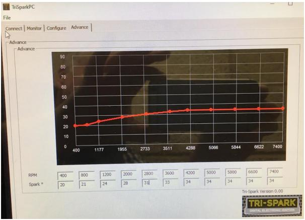
This proved to be a good starting point and the engine revved cleanly with stable tick-over and no propensity to kick-back.
